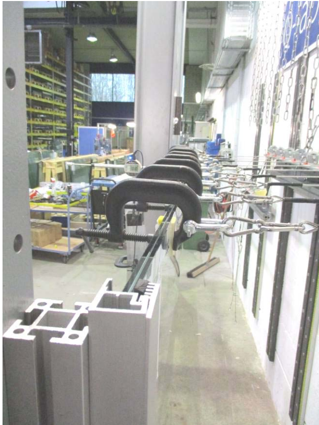
Resistance test on 2000 x 1100 mm., glass with external positioning.
