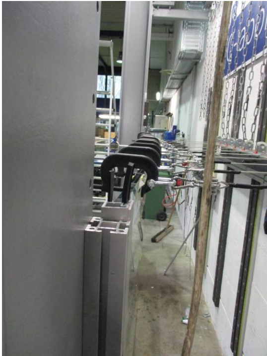
Resistance test on 2500 x 1100 mm., with internal positioning glass 8.8.82
