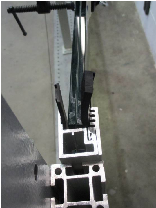
Resistance test on 3000 x 1100 mm., with internal positioning glass 8.8.2
