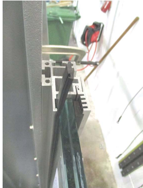
Resistance test on 2500 x 1100 mm., with internal positioning glass 8.8.82
